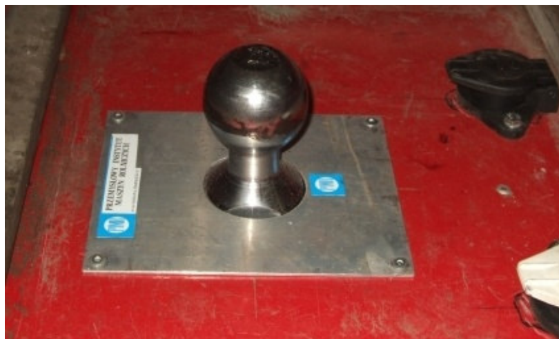
Figure 5. Land Rover Defender - 60mm hitch ball for coupling gooseneck trailer
