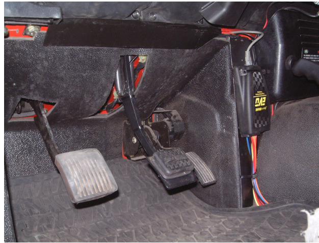
Figure 6. Brake Pad mounted on brake pedal and EVO controller on support plate.
