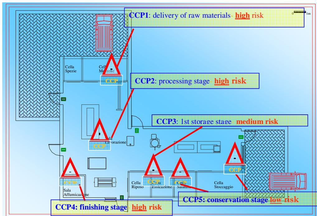
Figure 3. Critical points in the work cycle in a generic sausage factory
