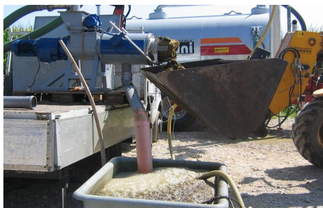
Figure 4. Separation of manure in liquid and solid portions with mechanical separator
