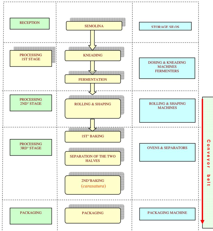
**Diagram 1. Functional areas, work cycle and plant engineering in a small bakery**
