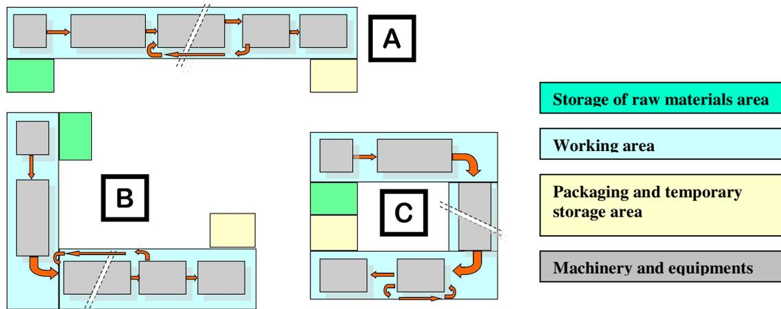
**Figure 1. Possible functional configurations: A linear; B "L"- shaped; C circular**
