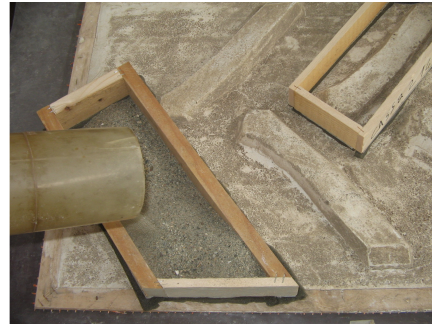
Figure 5. A volume sampler is filling with sand
