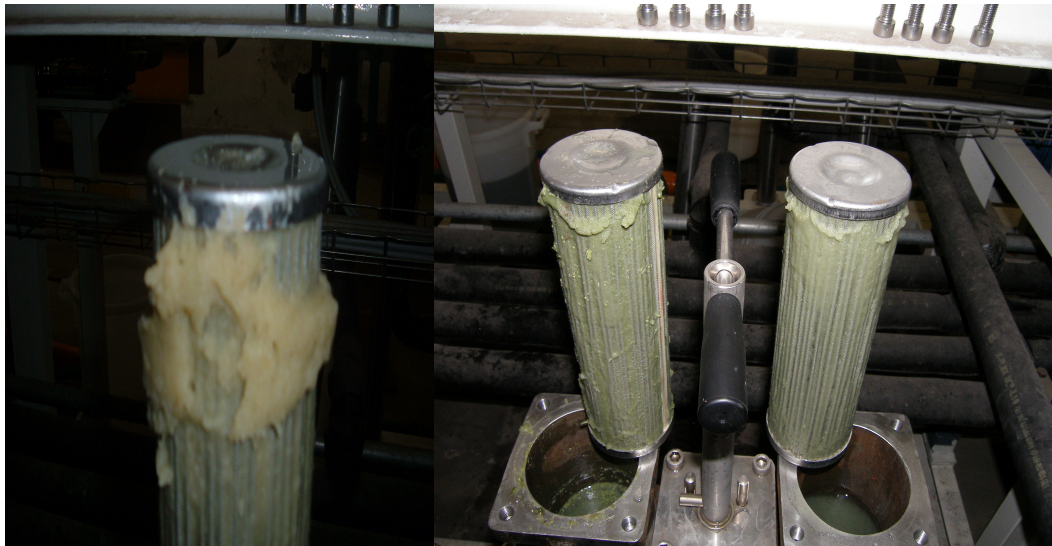
Figure 3. Cellulose cake formation in the twin 100 µm filters
