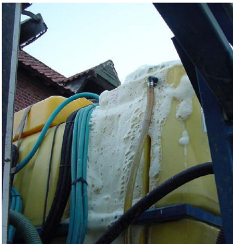
Figure 2. Example of accidental sprayer overfilling.
