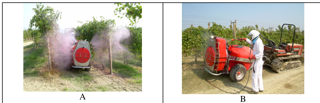
Figure 9. A) Application in the field of the diluted mixture obtained after the internal sprayer cleaning; B) external cleaning carried out in the field.
