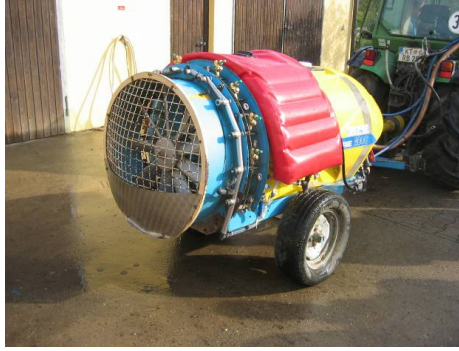
Figure 10. Sprayer equipped with an added auxiliary clear water tank.
