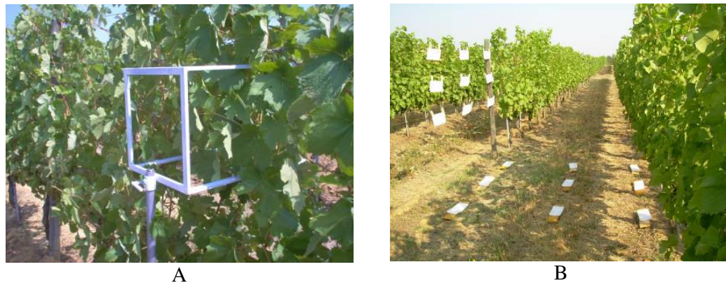
Figure 2. The iron frame used to define the portion of the row where to sample the sprayed leaves (A) and displacement of collectors on the ground and in correspondence of the second row to assess respectively ground losses and the amount of spray dispersed in the atmosphere beyond the treated row (B).
