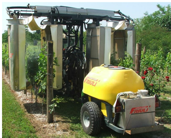
Figure 1. The prototype tunnel sprayer during application in the vineyard.
