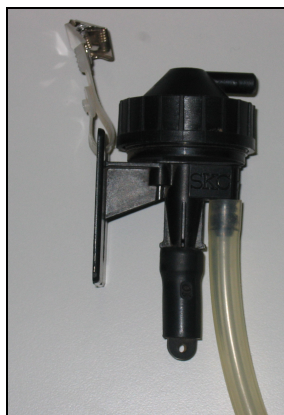
Figure 2. SKC cyclone for respirable fraction
