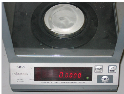
Figure 3. Analytical Gibertini scale
