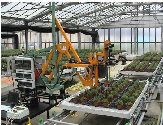
Figure 1. Fixed point robotic cell operating in the greenhouse.
