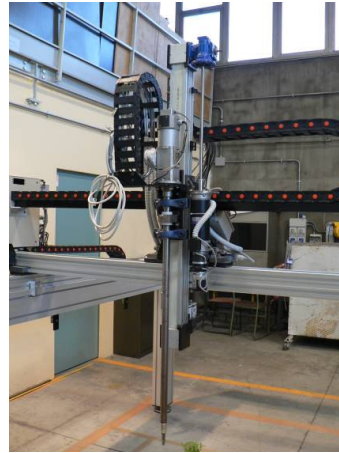
Figure 4. Cartesian robotic cell installed on the gantry structure. Figure 5. Detail of the fourth axis.
