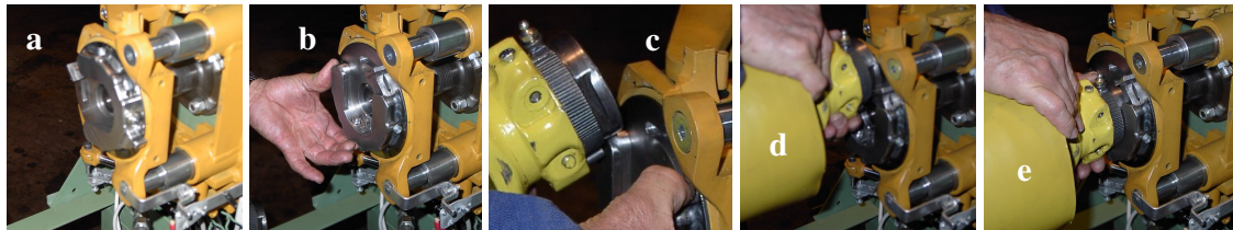
Figure 6. Operation sequence of the manual phase of the connection of the PTO-drive shaft to the MR-device
