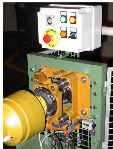
Figure 8. Test bench with the PTO-drive shaft connected and control board
