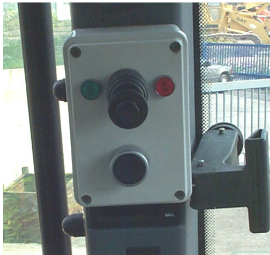
Figure 5. Control board on the cab of the tractor. G: green signal indicating the PTO-drive shaft engagement; R: red signal for the disengagement; J: joystick controlling the electro-hydraulic system; S: alarm turn-off
