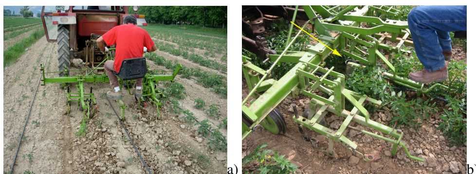
Figure 4. The precision hoe during an early intervention on processing tomato in 2007 (a). Detail of the "V" shaped tool utilized for the late hoeing intervention carried out in 2006 (b).
