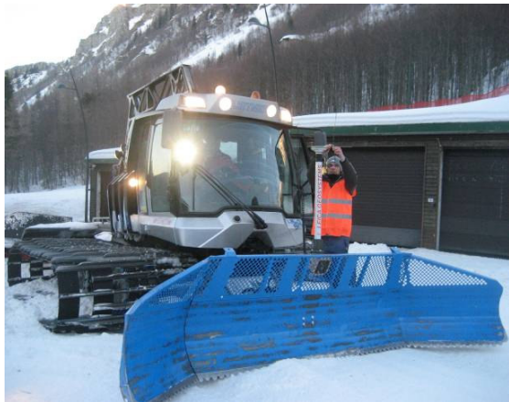
Figure 7. The snowgroomer Prinoth Everest equipped with the Leicageosystem Machine Automation System.
