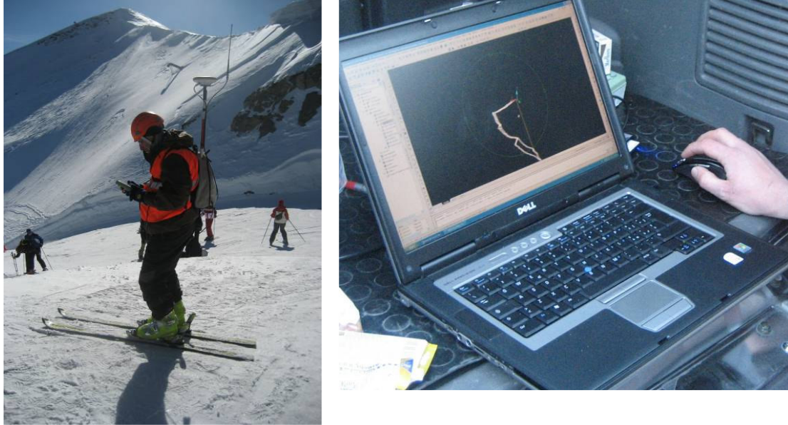
Figure 4. Points typing and the CAD georeferencing of the ski run
