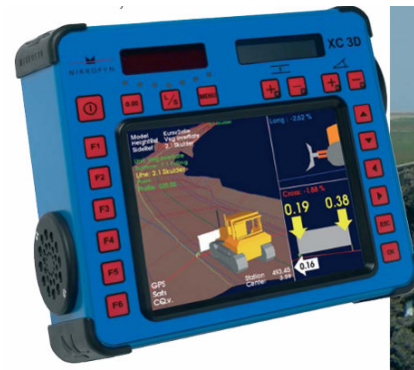
Figure 6. Information on the monitor of the DGPS Machine Automation System applied to an excavator making an half pipe
