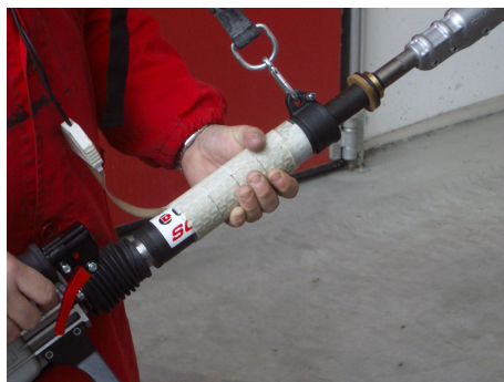
Figure 1. Matrix wrapper around the front olive shaker handlebar (left)
