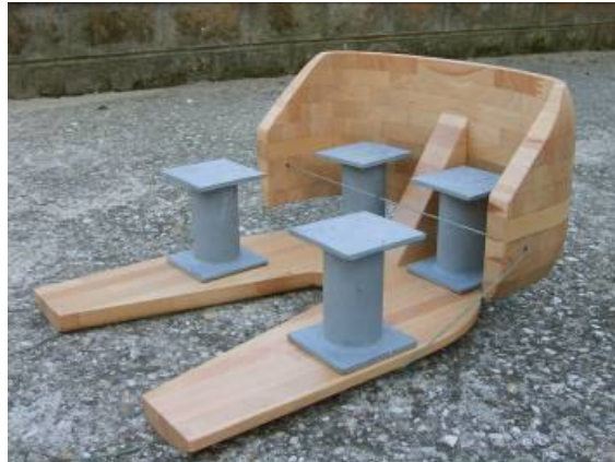
Figure 3. Instrument for the determination of the SIP complete with iron pedestals to support the weight
