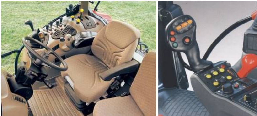
Figure 1. A tractor cabin guide and details of the joystick for traction command
