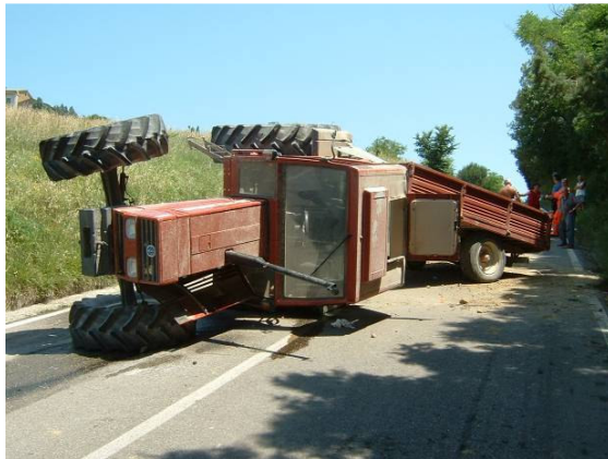
Figure 3. Accidents with conformed tractors equipped with ROPS and retention belt don't have heavy injuries for operators in almost all cases
