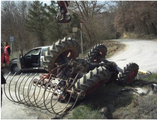
Figure 2. Old tractor without ROPS (Rollover Protective Structure) are cause of mortal accident. Inefficient brake system and lack of assisted-aid systems characterize these machines
