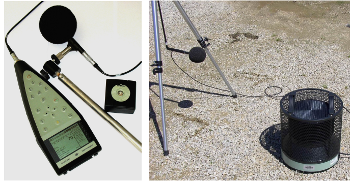
Figure 2. The real-time frequency analyzer, the microphone and the sound level calibrator (left); the reference sound source (right)
