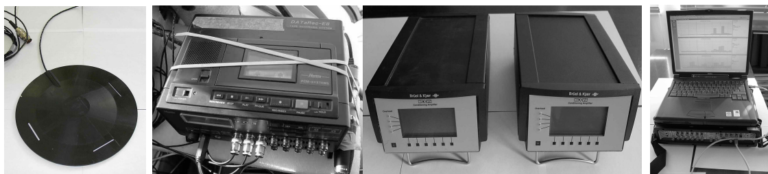
Figure 1. Instrumental chain A) triaxial accelerometer for driver seat; B) 8-channels digital recorder; C) 6-channell signal conditioners; D) "Pulse" data processing system
