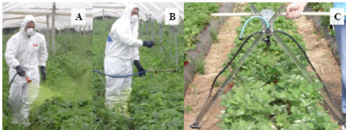
Figure 1. Tested hand held equipments: A - Spray gun; B - Boom segment; C - Adjustable row application kit
