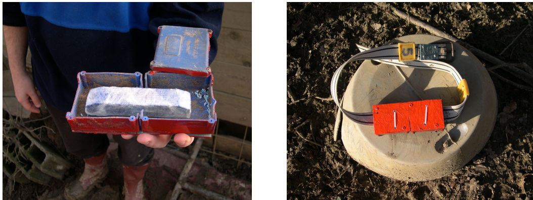
Figures 4 and 5. The active tag is put inside a plastic box and connected to a collar support to be fixed to the neck of the animal
