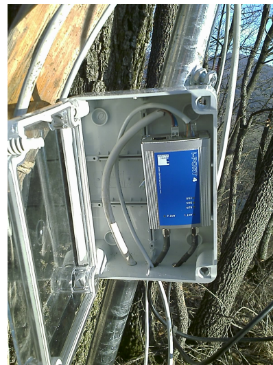
Figures 2 and 3. Installing antennas and reader for RFID system
