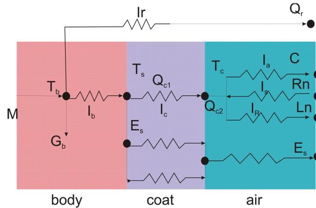
**Figure 2. Schematic diagram of modelled heat flows following McGovern and Bruce (2000)**
