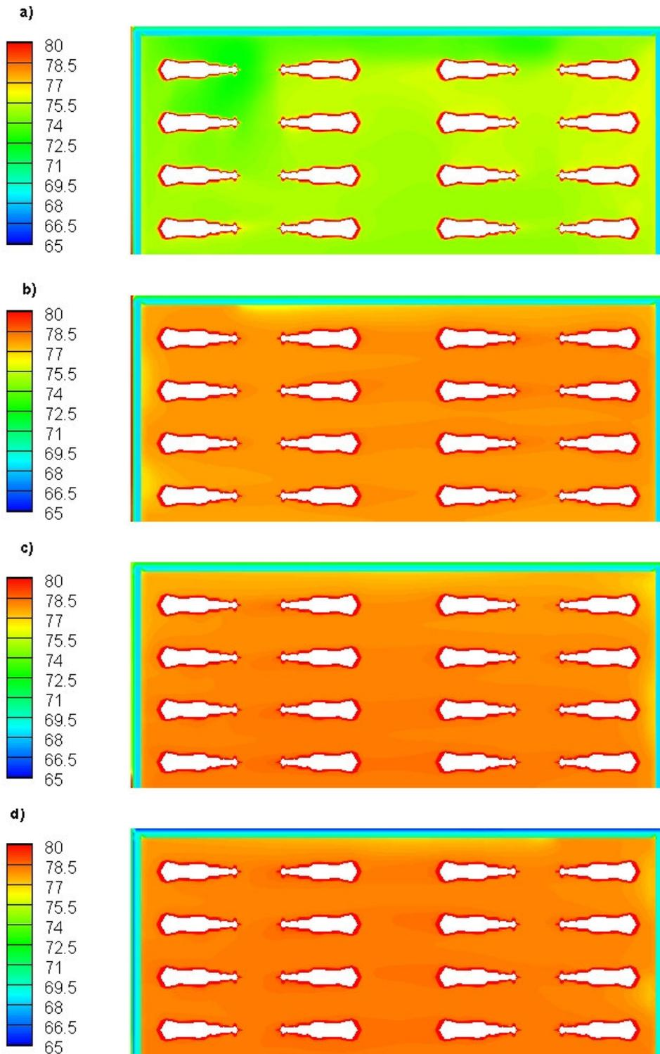
Figure 4. THI distribution for evaporative cooling panels positioned in: a) P1 b) P2 c) P3
