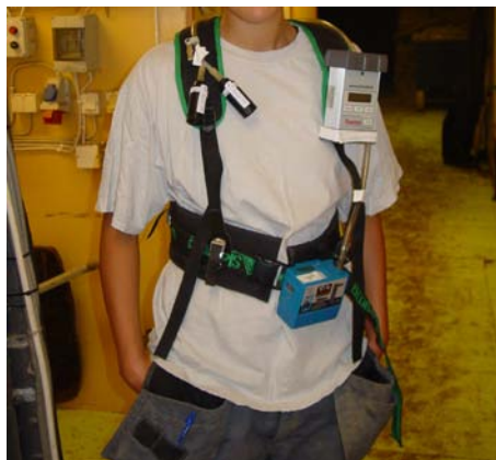
Figure 1. Instrument used for the personal sampling (a portable air pump that was connected with two sampling filters and the DataRAM).
