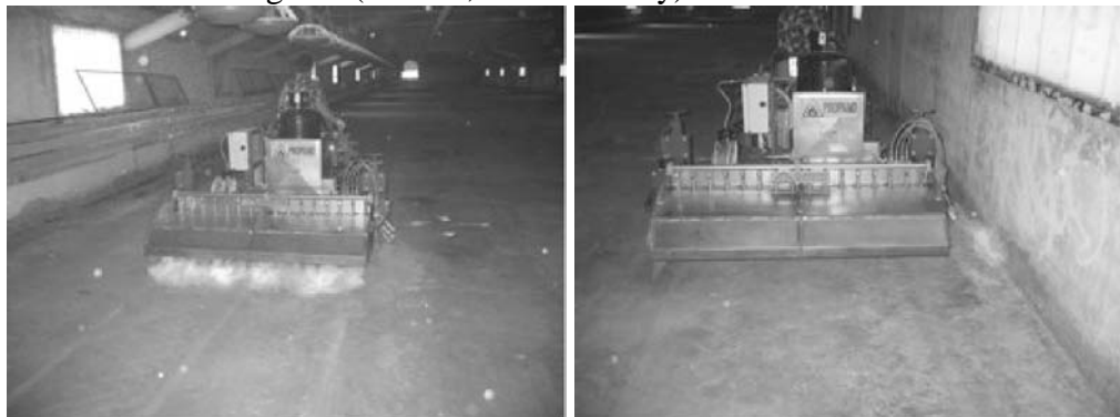
Figure 2. Flaming treatment in broiler house.
