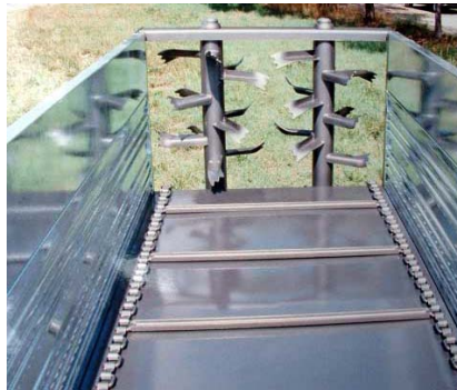
Figure 3. Example of manure spreader with vertical axes rotors rear spreading device
