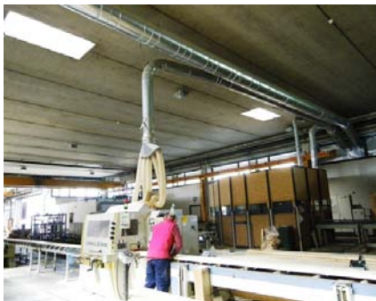
Figure 2. Particular of system of dust suction
