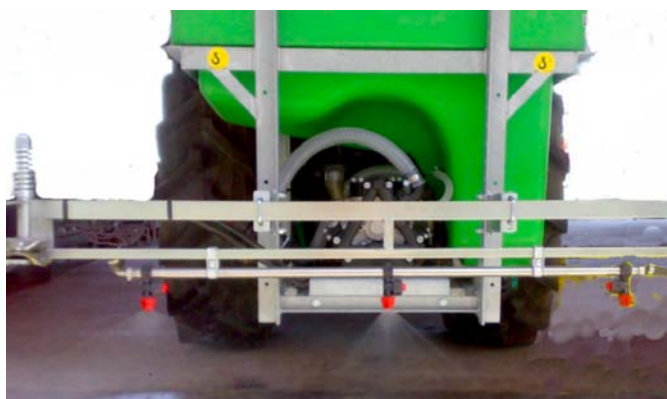
Figure 2. Boom sprayer used for the trials of resistance to agitation in the tank
