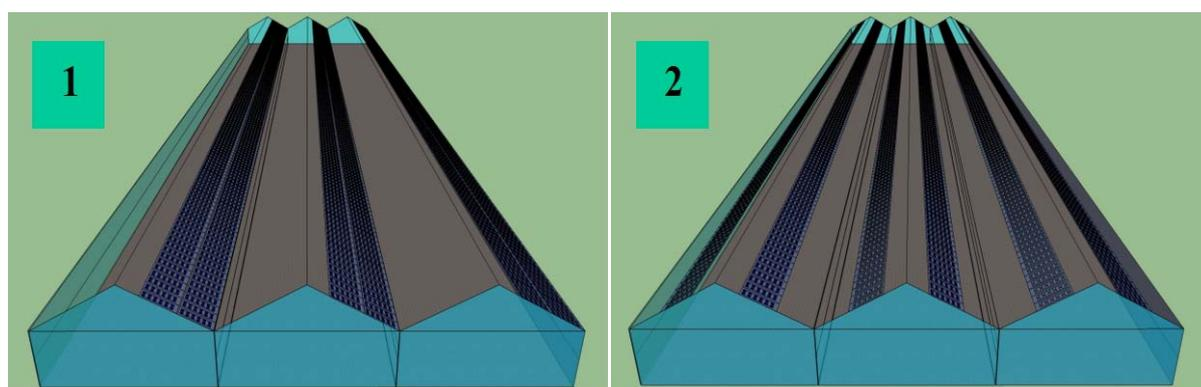
**Figure 2. PV generator placing: 1) PV modules installed on S oriented roofs as solution A and C. 2) PV modules installed by equally covering N and S roofs, as solution B and D. Shading level is 10% or 19% depending on the PV module used.**
